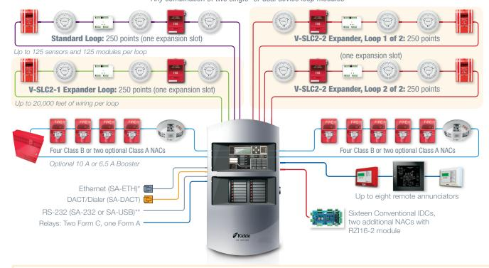
Each VS4 panel has room for up to two device loop controller modules in any combination of single or dual 250-device loops. VS4 comes with one loop that supports up to 125 detectors and 125 modules.
