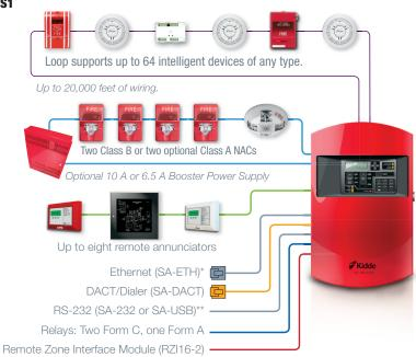
Each VS1 panel ships with one device loop controller that supports 64 devices of any type. This panel's device capacity cannot be expanded.
